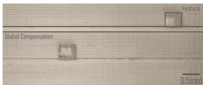
Fig. 9 | Global compensation method of Flui3d. A microscopic photograph from the side of a demonstrative 3D-printed microfluidic device utilizing global compensation with a slicing thickness of 50 \mu\text{m} .
