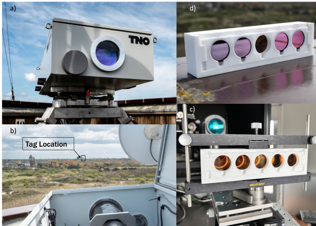
Fig. 4 | SLP field test setup. Mono-static OGS transceiver installed at location (a), free-space line of sight as seen from the Optical Ground Station transceiver location (b), SLP tag with unfiltered array of Corner Cube Retroreflectors installed in the support holder (c), example of a SLP tag with given combination of Band-Pass Filters (d). Pictures courtesy of Eric de Vries.
