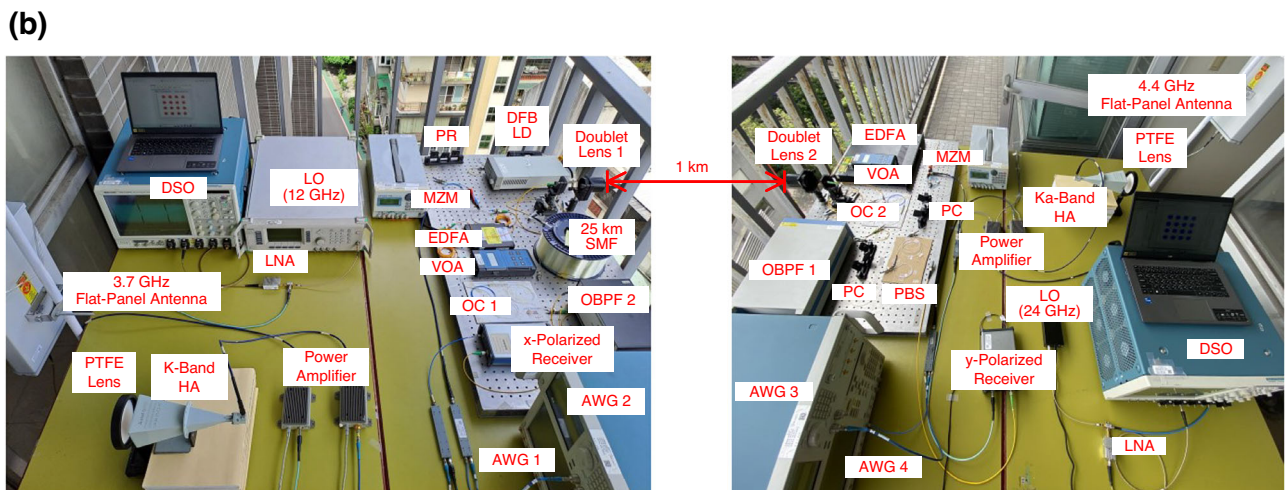
Fig. 5 5G (5G, fifth-generation) MMW (MMW, millimetre-wave)/sub-6 GHz signals through two-way fibre-FSO (FSO, free-space optics)-wireless communications. a Architecture of 5G MMW/sub-6 GHz signals through two-way fibre-FSO-wireless communications employing polarisation-orthogonal modulation technique. b A photo of experimental setup. DFB LD distributed feedback laser diode, PR polarisation rotator, 16-QAM-OFDM 16-quadrature amplitude modulation-orthogonal frequency-division multiplexing, MZM Mach-Zehnder modulator, EDFA erbium-doped fibre amplifier, VOA variable optical attenuator, OC optical circulator, SMF single-mode fibre, OBPF optical band-pass filter, PC polarisation controller, PBS polarisation beam splitter, PA power amplifier, PTFE polytetrafluoroethylene, HA horn antenna, LO local oscillator, LNA low noise amplifier, DSO digital sampling oscilloscope.
