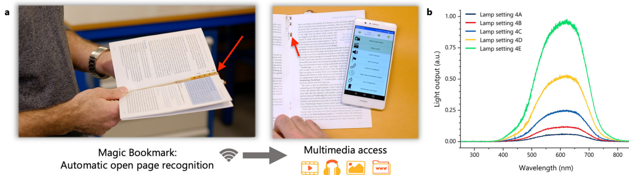
Fig. 1 The augmented paper ecosystem and the test conditions. a Overview of the Magic Bookmark ecosystem; an electronically augmented bookmark is used on a printed book to automatically detect and transmit the open page to an adjunct device. b The emission spectrum of the microscope lamp that is used to assess the suitability of the developed photodetectors (settings refer to the lamp settings as outlined in Supplementary Table 1).
