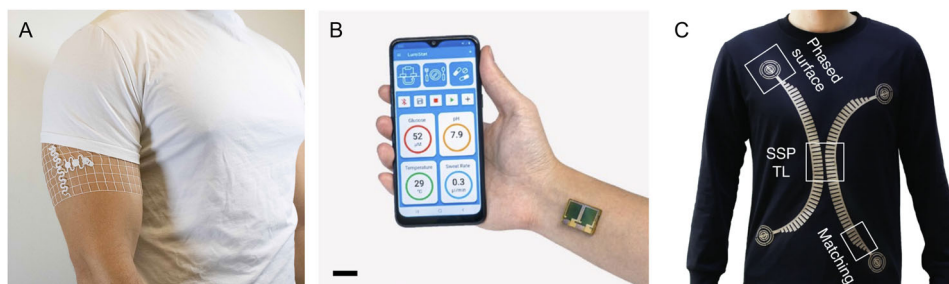
Fig. 3 Comparison of wirelessly recharged or powered wearables. A Biosymbiotic device with a small battery and recharge at distance 22 , enabling 24/7 operation without user interaction, image credit Gutruf lab. B Photonically powered device via perovskite solar cells enabling operation during light hours without additional infrastructure, Reproduced with permission from ref. 24 , copyright (Springer Nature BV, 2023) C Wireless power distribution via textile 25 enabling operation utilizing the smartphone as a power source.
