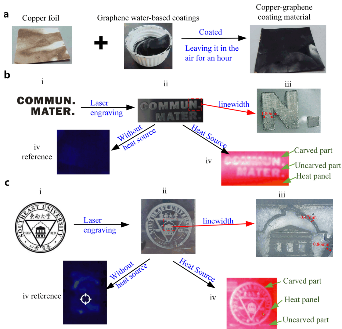
Fig. 1 The processes of the CGC materials, CM logo, and SEU logo surfaces. a The schematic of CGC materials. b (i) Selection a CM logo; (ii) Engraving the CGC material through CO 2 laser engraving machine to form the CM logo surface; (iii) Zooming in the red dashed box of CM logo surface to observe the detail of the processing and measure the linewidth through the electronic magnifying glass; The linewidth of char “N” is 1.80 mm; (iv and iv reference) Taking photos using an IR camera with and without heat source. c (i) Selection a complex logo; (ii) Engraving the CGC material through CO 2 laser engraving machine to form the SEU logo surface; (iii) (iii) Zooming in the red dashed box of the SEU logo surface to observe the smoothness of the curve and measure the linewidth; The linewidth of the curve and bold straight line are the 0.47 and 0.86 mm; (iv and iv reference) Taking photos of the SEU using an IR camera with and without attaching to the surface of heat source.
