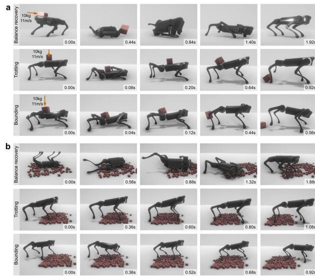
Extended Data Fig. 6 | Robustness tests of key-state policies for balance recovery, trotting and bounding against unexpected perturbations. a, Perturbation by a 10 kg flying box at 11 \text{ m s}^{-1} initial velocity for balance recovery (top), trotting (middle) and bounding (bottom). b, Stable traversal over unseen rubble for balance recovery (top), trotting (middle) and bounding (bottom).
