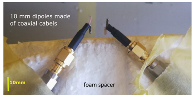
Fig. 4 Photo of the electric dipoles used in the experiments. The 10 mm dipoles are made from a coaxial cable and fixed on the foam spacer.
