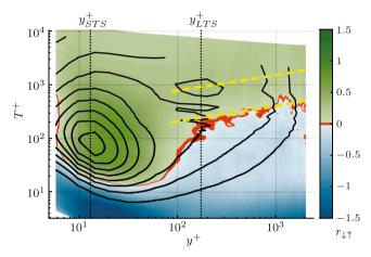
**Fig. 5 Scale-dependent results for the turbulent channel flow.** Colored areas corresponds to the ratio  $r_{\downarrow\uparrow}$ , while the black contours refers to the pre-multiplied energy spectra  $\phi_{uu}^+$  (contour level range 0.25-2, level step 0.25). The two yellow dashed lines refer to the  $\lambda_x^+ \sim y^{+3/7}$  scaling<sup>59</sup>, in terms of time scales  $T^+ = \lambda_x^+/U^+$ .
