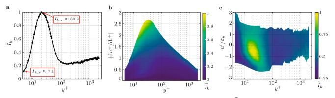
**Fig. 4 Full-signal time irreversibility (TI) results for the turbulent channel flow. a** Wall-normal behavior of  $\tilde{l}_k$ . The maximum and minimum values of the irreversibility ratio  $l_{k,r}$  are also highlighted. Conditional analysis of  $\tilde{l}_k$  with respect to  $y^+$  and **b** the local signal slope  $|du^+/dt^+| = U^+|du^+/dx^+|$ , and **c**  $u'/\sigma_u$ . Intervals of  $|du^+/dt^+|$  and  $u'/\sigma_u$  are binned as 2: 2: 100 percentiles.
