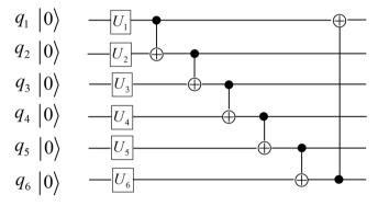
**Fig. 5 The 1st example of the hardware-efficient ansatz.** The figure shows the quantum circuit of one layer of the hardware-efficient ansatz in ref. <sup>33</sup>  $U_1$  through  $U_6$  are 1-qubit unitaries applied to the qubits  $q_1$  through  $q_6$ , respectively. The CNOT gate layer then copies the unitary dependencies around the qubits. The final unitary dependence picture as described in Eq. (10) shows the qubits are highly-dependent on manipulations and measurement statistics.
