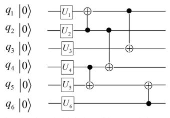
**Fig. 6 The 2nd example of the hardware-efficient ansatz.** The figure shows the quantum circuit of one layer of the hardware-efficient ansatz in ref. <sup>34</sup>  $U_1$  through  $U_6$  are 1-qubit unitaries applied to the qubits  $q_1$  through  $q_6$ , respectively. The CNOT gate layer then copies the unitary dependencies around the qubits. The final unitary dependence picture as described in Eq. (11) shows the qubits are more independent in manipulations and measurement statistics.
