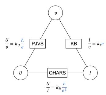
**Fig. 4 The metrology triangle.** The metrology triangle involving the Kibble balance (KB), and two quantum standards : the programmable Josephson voltage standard (PJVS), and the Quantum Hall array resistance standards (QHARS). For the measurement presented here, the nominal values of the scaling factors for the 100 g mass are  $k_R = 1/26$ ,  $k_U = 18,350$ , and  $k_I = 477,100$ .
