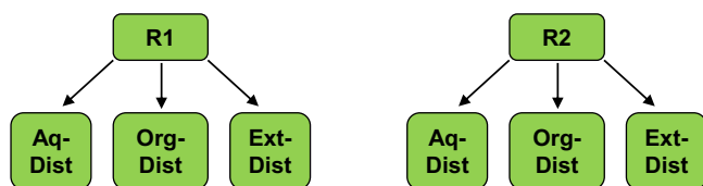
Fig. 8 Process variants for the production of 4,5-dimethyl-1,3-dioxolane. Six process variants are compared. Two general process routes (R1 and R2) with three downstream concepts (distillation from aqueous solvent: DIST-AQ, distillation from MARS: DIST-ORG, extraction into aqueous solvent: EXT-DIST) are investigated.
