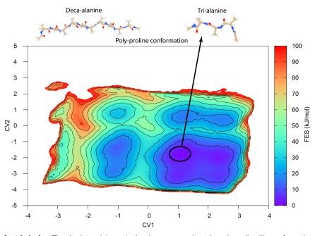
**Fig. 5 Free-energy surface for tri-alanine.** The absolute minimum in the plot corresponds to the poly-proline-like conformation, which is not the preferred conformation in the case of deca-alanine, represented in the upper left corner.
