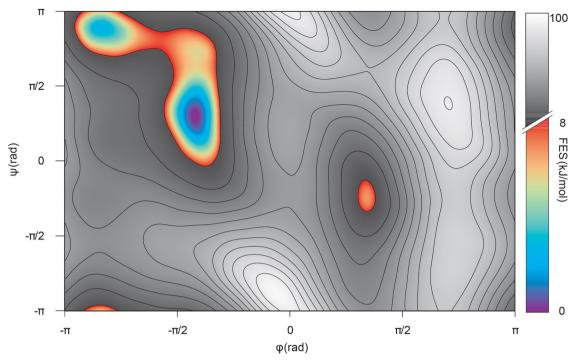
Fig. 2 Free-energy surface for the conformational space of alanine dipeptide. In the color range the interval from 0 to 8 kJ/mol is employed for the threshold. The rest of the surface represents high-energy conformations that have been grayed out.
