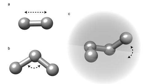
Fig. 9 Representations of various constraints in MD simulations. Graphical representation of the bond (a), angle (b), and dihedral angle (c) constraints in defining a molecule in MD simulations.
