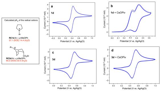
Fig. 13 Electrochemical study. Cyclic voltammograms of N-p-methoxyphenylamines 1d and 3d (1 mM) in the absence (a and c) and in the presence of cesium pivalate (1.2 mM) (b and d). Voltammograms were recorded at 100 mV/s in acetonitrile containing [Bu<sub>4</sub>N][PF<sub>6</sub>] (0.1 M) as a supporting electrolyte.  $pK_a$ s are indicated in red. Voltammogram traces are depicted in blue.
