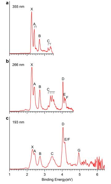
**Fig. 1 Photoelectron spectra of PbB<sub>2</sub>O<sup>-</sup>. a** At 355 nm. **b** At 266 nm. **c** At 193 nm. The vertical lines represent resolved vibrational progressions.
