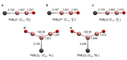
**Fig. 3 Global minimum structures of PbB<sub>2</sub>O and PbB<sub>3</sub>O<sub>2</sub> at different charge states. a** PbB<sub>2</sub>O<sup>-</sup>. **b** PbB<sub>2</sub>O<sup>2-</sup>. **c** PbB<sub>3</sub>O<sub>2</sub><sup>-</sup>. **e** Pb
