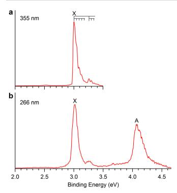
Fig. 2 Photoelectron spectra of PbB<sub>3</sub>O<sub>2</sub>-. a At 355 nm. b At 266 nm. The vertical lines represent resolved vibrational progressions.
