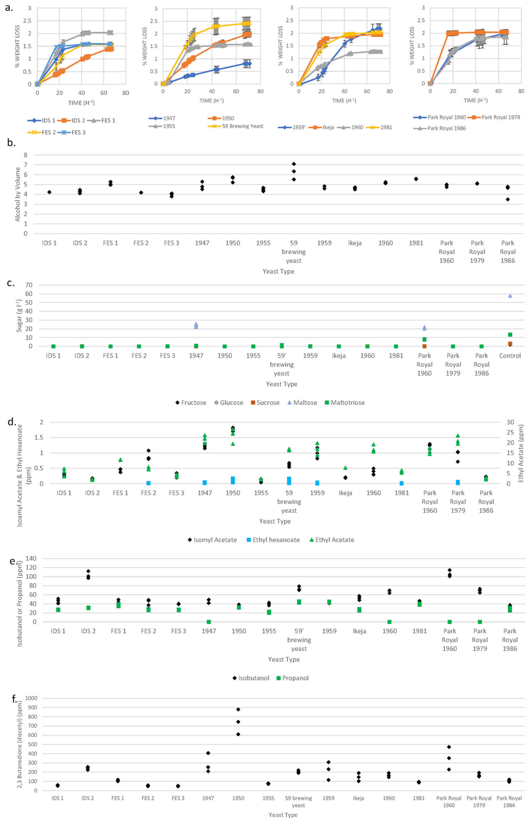
Fig. 4 Phenotypic assessment of the Guinness yeast. a Percentage weight loss, b ethanol production, c sugar concentration d assessment of esters, e higher alcohols and f 2, 3 butanedione (diacetyl) production at the cessation of fermentation using the different Guinness yeast. Fermentations were performed using 100 ml of 12°P all-malt wort, with an inoculation rate of 1 \times 10^7 ml -1 cells. Samples were incubated at 25 °C and stirred at 250 rpm. Observations presented are n = 3 biologically independent experiments. In a each time point represents the mean of 3 independent replicates and standard errors are shown as SD \pm error bars.
