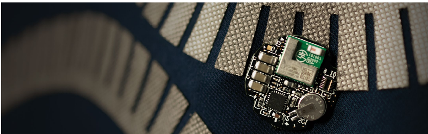
Photograph of a wirelessly powered Bluetooth module that is placed on a metasurface fabricated from a conductive textile. The metasurface can be used to connect wearable sensors around the body 3 . Credit: Xi Tian, National University of Singapore.
