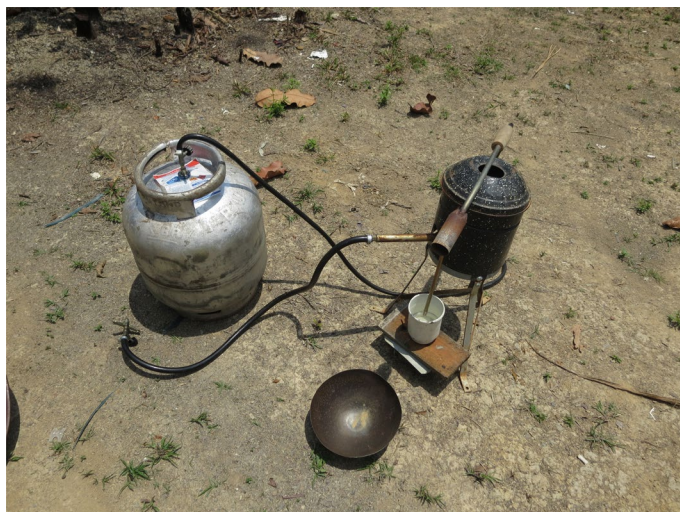
Fig. 2 | A typical retort. Photograph shows a typical retort as used in the Tapajós region.
