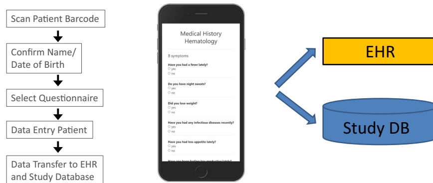
Fig. 6 EDC workflow with EHR integration. Patient barcode is scanned with an iPad to identify the patient. After confirmation of patient’s name and date of birth, a suitable questionnaire is selected and the iPad is handed to the patient for data entry. When data collection is completed, data are transferred simultaneously into EHR system and into study database.
