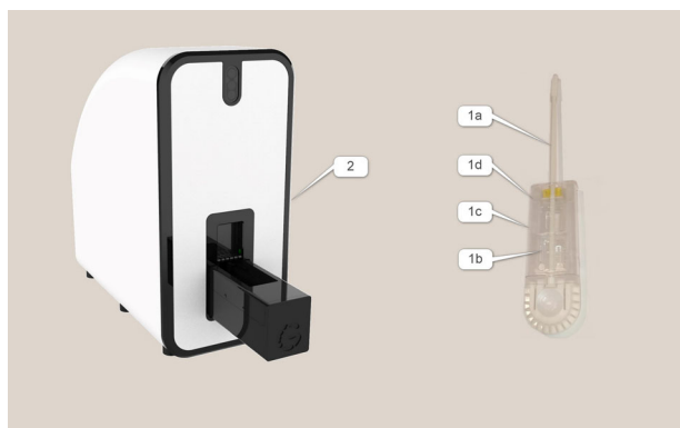
Fig. 4 The Gyni investigational test system components. Actual hardware components of the disposable discharge collection tool and the tabletop scanner.
