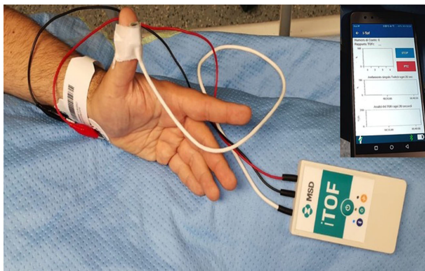
Fig. 1 The i-TOF Device. The i-TOF device consists of a triaxial accelerometer, two poles for nerve stimulation, and wireless connection on a smartphone by application.
