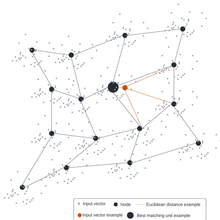
Fig. 9 Schematic diagram of SOM analysis. a Flowchart of SOM algorithm and b concept diagram of SOM.
