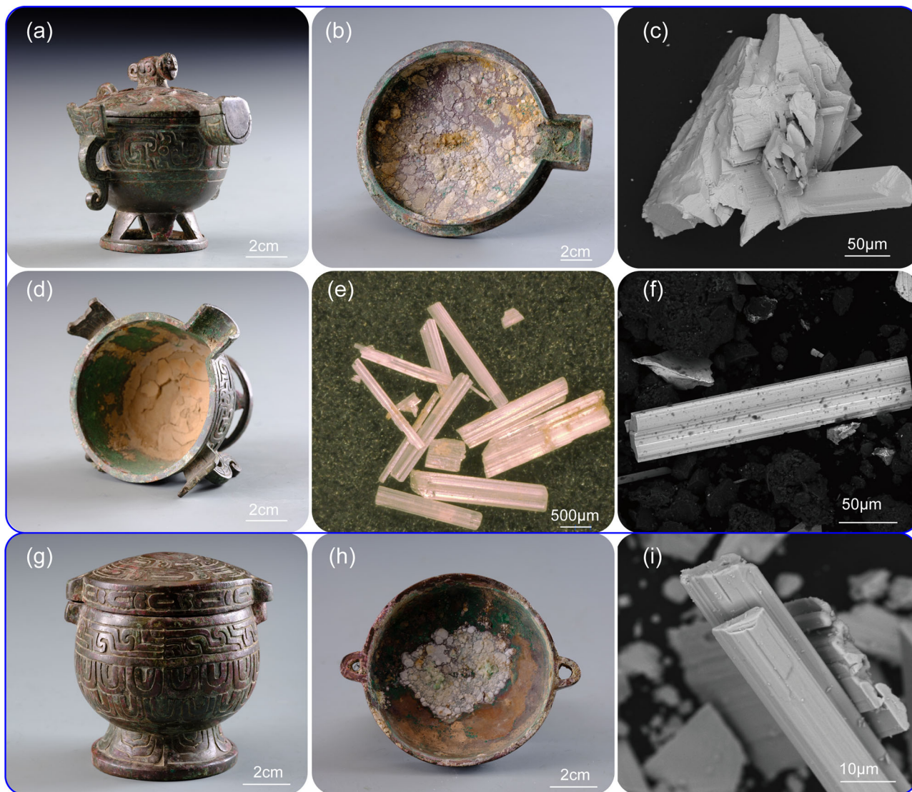
Fig. 4 Some cosmetic bronze containers in Liangdaicun site and lead white residue inside. a The miniature bronze container of Fu (code M26:138); b the white residue (LW-1a) on its lid; c the SEM observation of sample LW-1a with multiple stacks layout; d numerous pure lead white residue particles scattered within the soil off the bottom of M26:138; e some elongated needles and prismatic lead white (LW-1c) gently separated from the soil of d ; f the SEM observation of sample LW-1c; g the miniature bronze container of round-foot jar (code M26:137); h the white residue (LW-2a) on its lid; i the SEM observation of sample LW-2a with prismatic shape.
