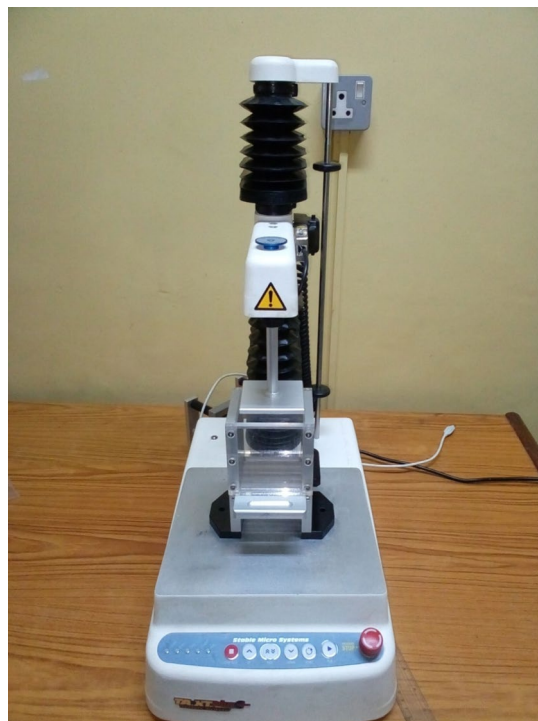
Figure 2. A picture of the texture analyzer. Source: Maziya-Dixon et al. (2023) (Next Gen report).
