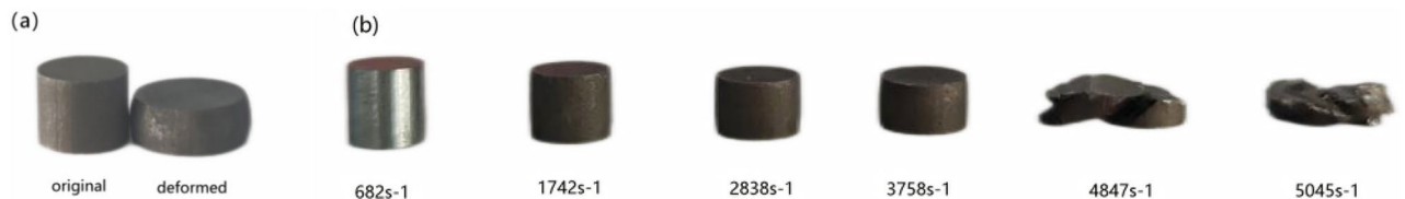
Figure 4. Comparison of the original and deformed specimens: a Quasi-static compression test, b SHPB tests.
