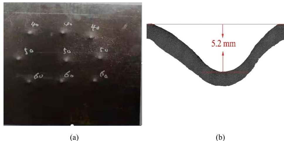
Figure 2. Appearance of the target plate after the shooting test: a the back, b the crater depth of Test-3.
