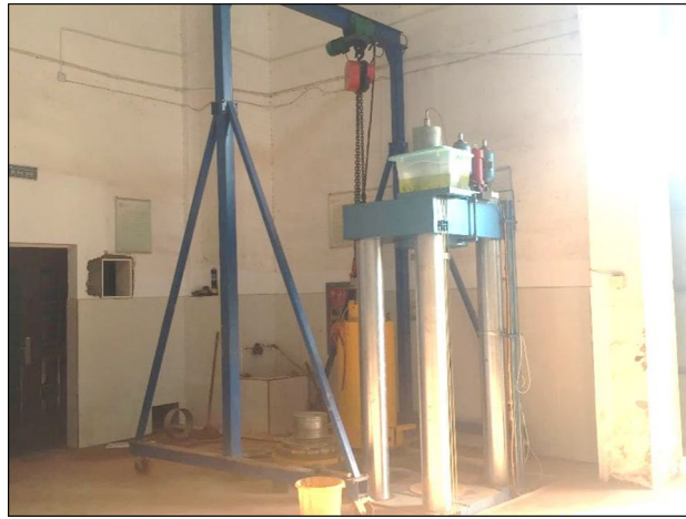
Figure 2. The large-scale dynamic and static triaxial apparatus.
