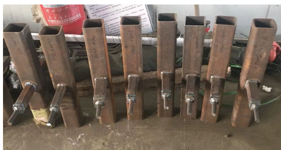
(a) chord and brace were welded together
