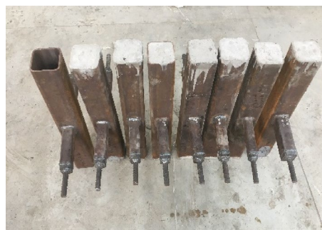
(c) Concrete was cured for 28d
