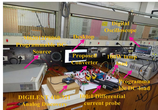
Figure 11. Introduced power conversion circuit testing network.
