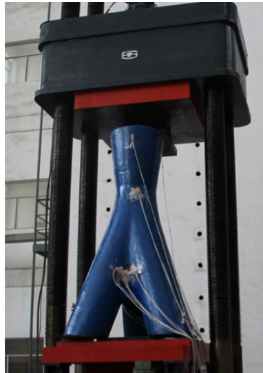
Figure 5. Test-specimen and loading device for the experiment.
