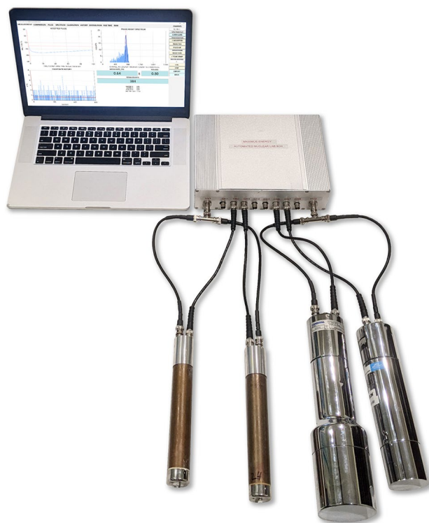
Figure 1. The Automated Nuclear Lab system: sample configuration with two ^3\text{He} proportional neutron counters and two NaI(Tl) gamma scintillation detectors.
