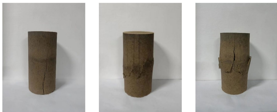
(a) Xanthan gum content 0% (b) Xanthan gum content 1.5% (c) Xanthan gum content 3%
