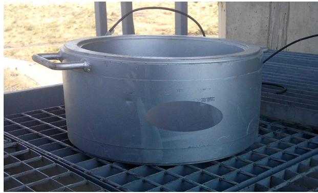
Figure 12. Example of a load cell to control the total stress experienced by the stay cables of a bridge.
