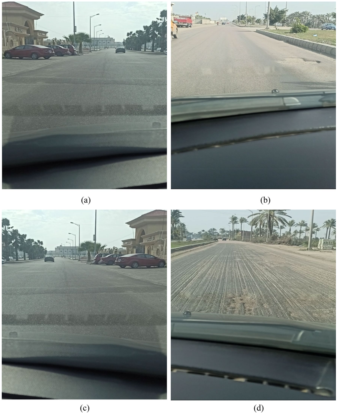
Figure 2. Representative data samples for different road conditions. (a) Normal road, (b) Pothole, (c) Speedbump, (d) Bad road.
