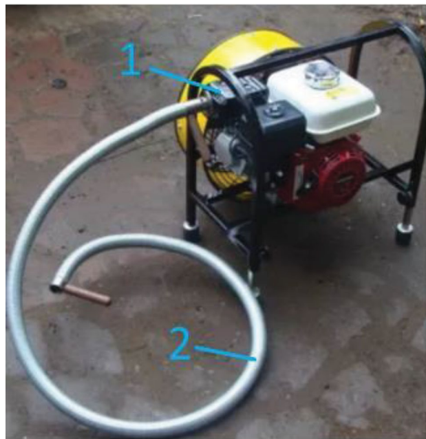
Figure 5. Rescue ventilator with exhaust system from the combustion engine, where: 1—exhaust manifold with silencer, 2—exhaust gas duct.
