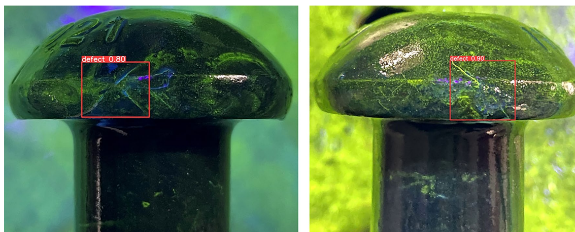
Figure 17. The results of detecting discontinuous cracks by decentralized target center and low overlap rate labeling method.
