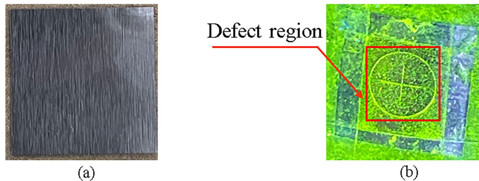
Figure 4. Experimental verification of composite magnetization effect with (a) Test piece before composite magnetization, (b) “Cross” fluorescent magnetic trace.
