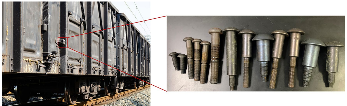
Figure 1. Defective rivets for train parts.
