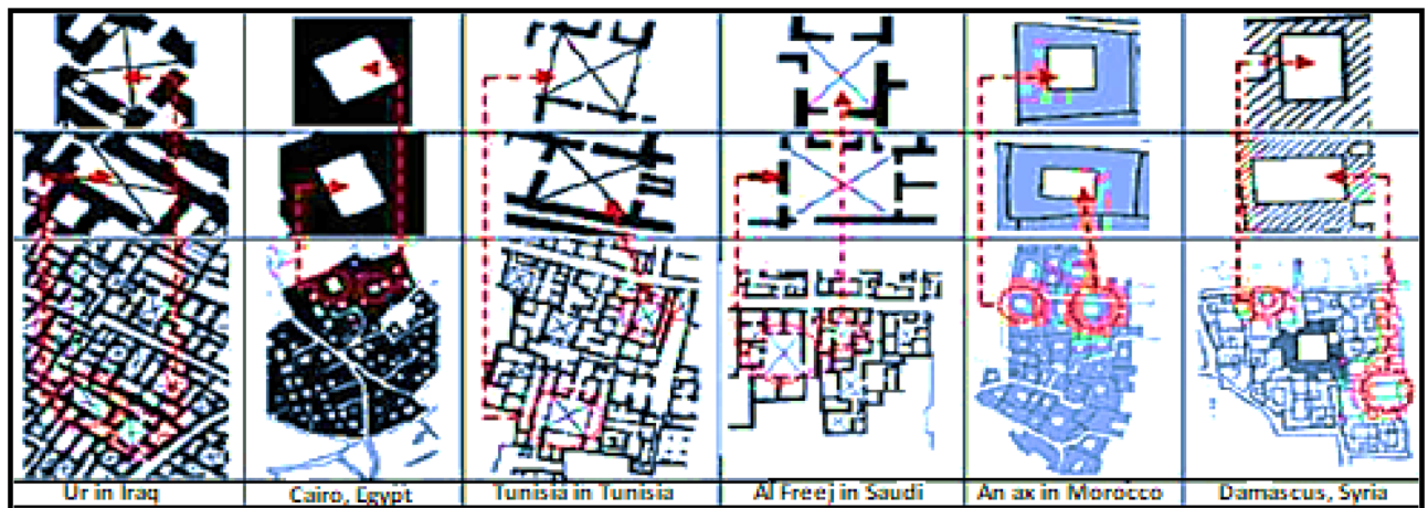
Figure 3. The prevailing formation of the courtyard in heritage buildings that diversifies between square and rectangular shapes 11 .
