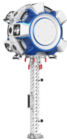
Figure 1. Tunnel surface information detection subunit.
