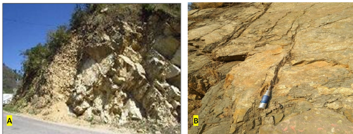
Figure 3. Exposure of the rock outcrop in the study area; (A) Berinag quartzite outcrop exposure, (B) massive quartz arenites outcropping with a moderate fracturing.
