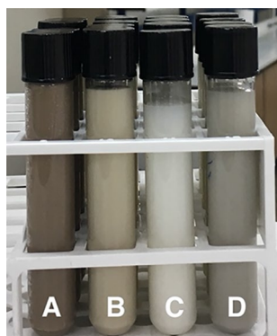
Figure 5. Colors of 3% (w/w) suspensions of 3.4% (w/w) silver-incorporated geopolymer powders. A, B, C, and D denote suspensions of the powders after synthesis and after calcination at 550 °C, 850 °C, and 1050 °C, respectively.
