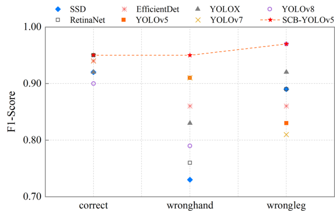
Figure 8. The F1-SCORE of detectors, where SCB-YOLOv5 has the highest F1-SCORE, while the other detectors exhibit less favorable detection results for the classification of wronghand, again confirming Table 2 above.
