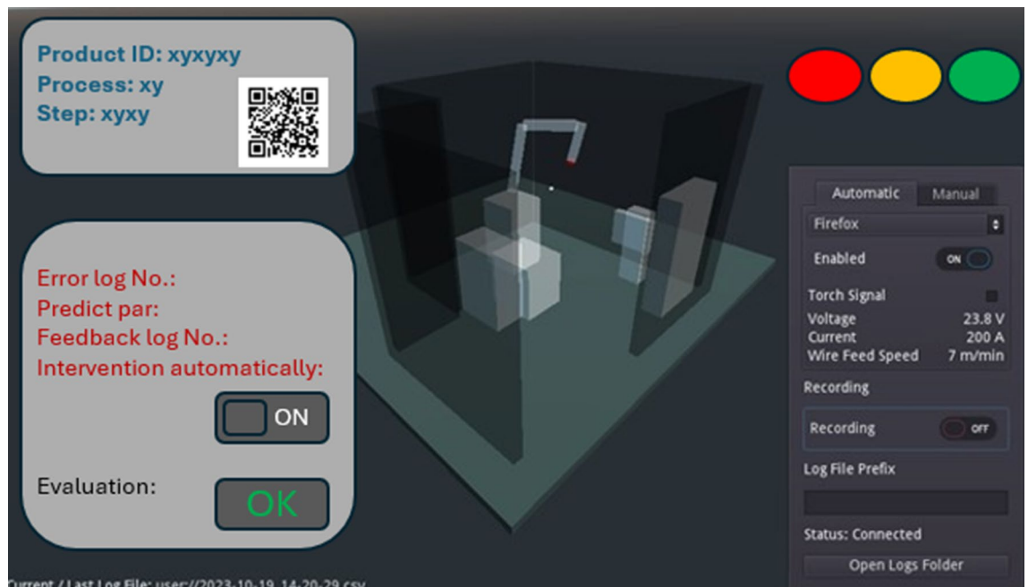
Figure 9. A possible digital interface design example for the use of digital twins.
