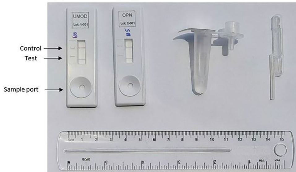
Figure 4. Lateral flow device assembly kit for urinary biomarkers Uromodulin (UMOD) and Osteopontin (OPN). (Left to Right) Biotin/Polystreptavidin (PSA) based LFD for UMOD, Standard LFD for OPN, Diluent tube and Disposable pipette.
