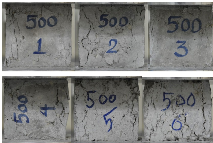
Figure 7. Cracks and brittleness of samples exposed to 500 °C temperature under pressure test.
