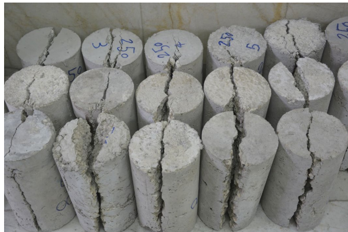
Figure 12. Cracks and fractures of samples under tensile test.
