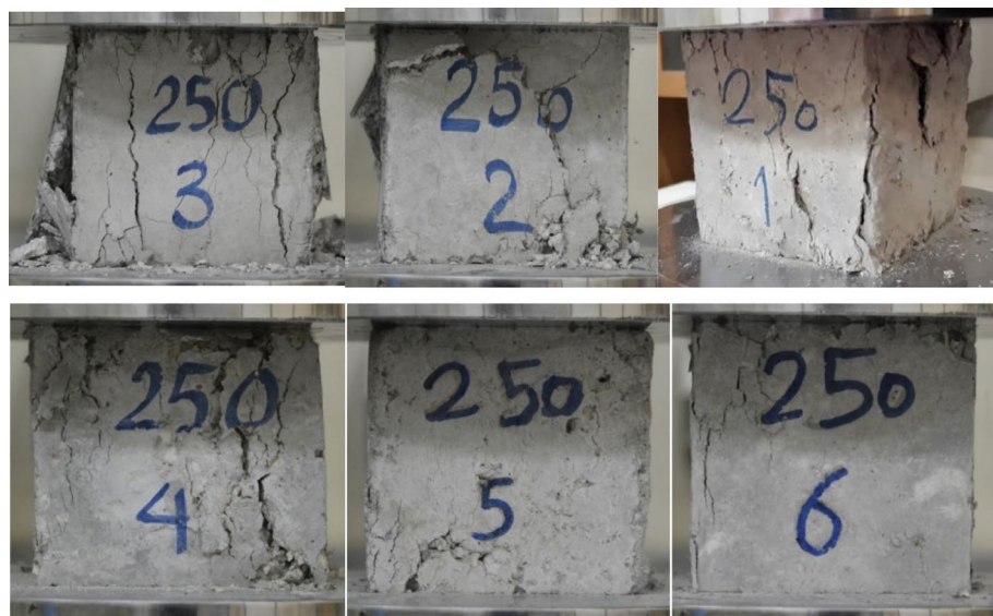
Figure 6. Cracks and brittleness of samples exposed to 250 °C temperature under pressure test.
