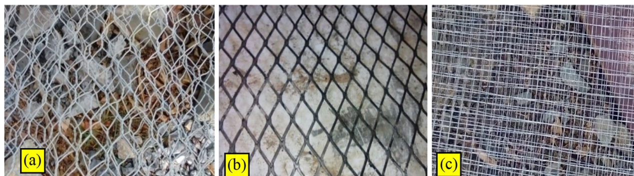
Figure 3. Different types of mesh (a) Hexagonal (chicken) wire mesh, (b) Welded square wire mesh (c) Expanded metal mesh.
