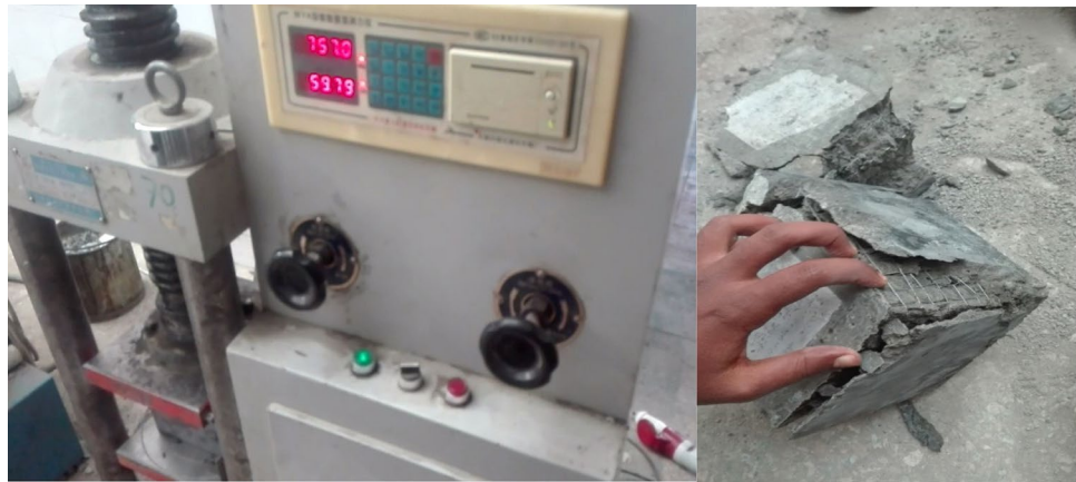
Figure 10. Testing of cube specimen.
