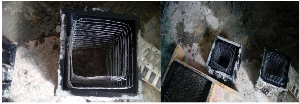
Figure 9. Cubes prepared before concrete casting.
