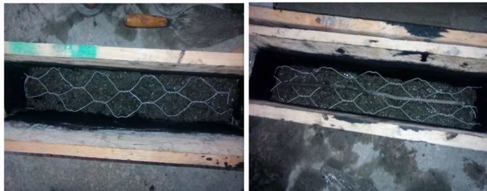
Figure 5. Casting of ferro concrete beam model using hexagonal (chicken) wire mesh.
