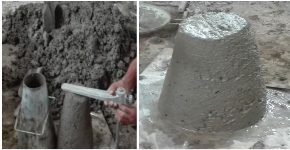
Figure 4. Workability test of concrete.
