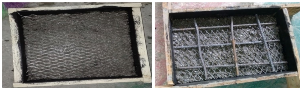
Figure 11. Slab specimens prepared for casting and during casting.
