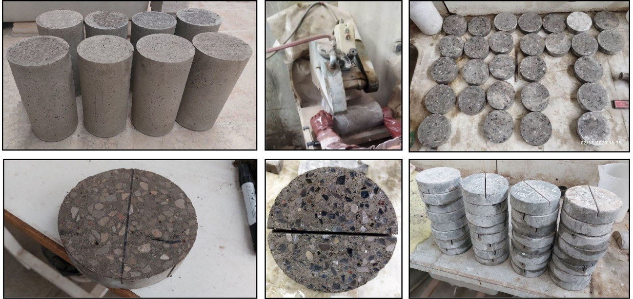
Figure 4. Process of ENDB specimen preparation.
