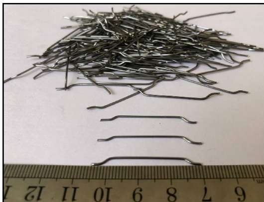
Figure 2. Hooked-end steel fiber.
