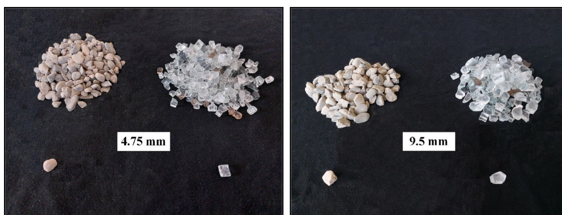
Figure 1. Coarse aggregates of NCA and WGCA used for casting SFR-SCC mixtures.
