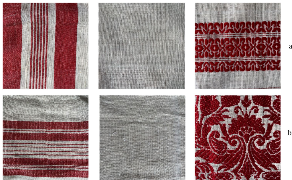
Figure 4. Images acquired of the two loom type of the “gamucha” (a handloom; b powerloom).
