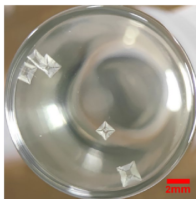
Figure 3. Crystals in the bottom view of vials induced by laser with the effect of 19 wt% PAA.
