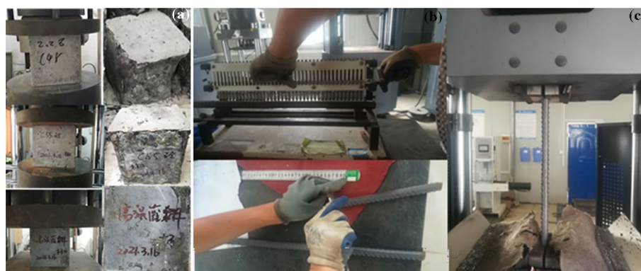
Figure 4. (a) Compressive test of concrete; (b) tensile test of compression test.
