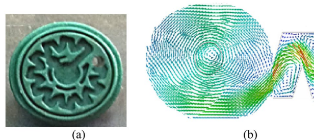
Figure 3. Water path map (a) and velocity vortex profile (b) in the outlet area of the emitter.
