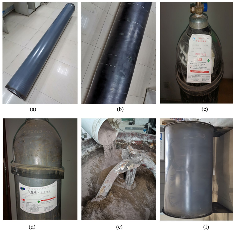
Figure 6. Experimental materials. (a) Inner steel cylinder; (b) Rubber airbag; (c) Air; (d) CO 2 ; (e) Soil mixture; (f) External steel cylinder.
